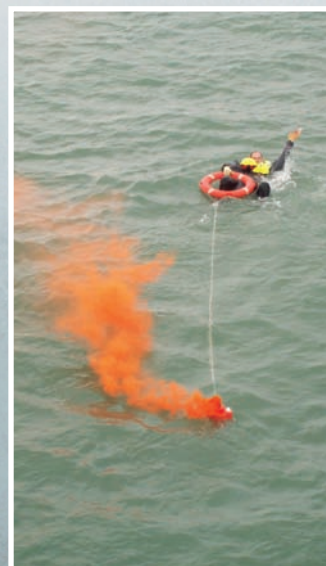
Light & Smoke signal attached to Lifebuoy indicates position of the man overboard to the ship's helmsman by day or night
